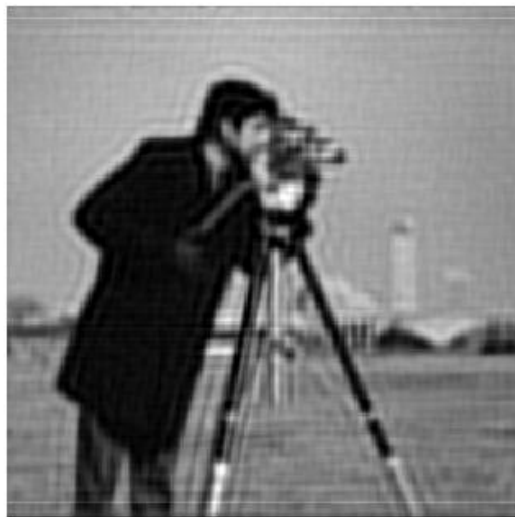
Figure 60: Result of Figure 2 restored by a direct Wiener filter, \text{ISNR} = 2.6 \text{ dB}
