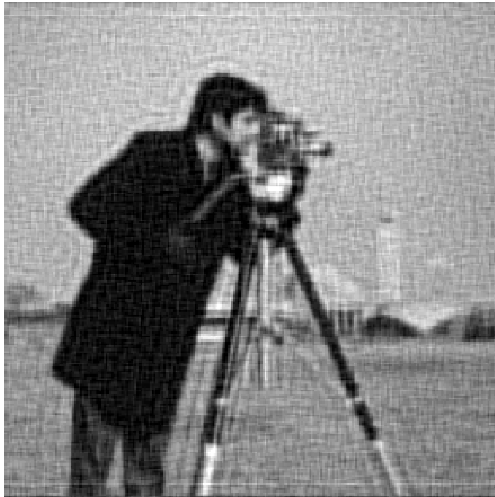
Figure 51: Result of Figure 3 restored by the iterative Tikhonov-Miller algorithm after 20 iterations, \alpha = 10^{-2} , ISNR = 0.23 dB
