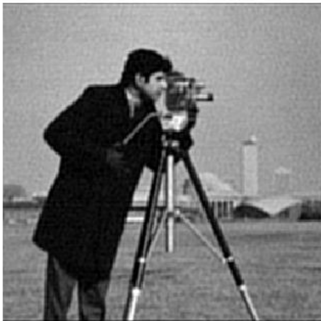
Figure 63: Result of Figure 5 restored by a direct Wiener filter, \text{ISNR} = 1.0 \text{ dB}
