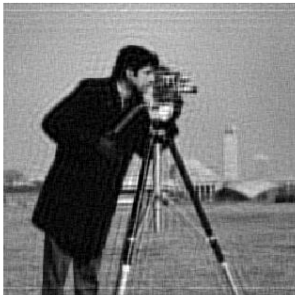
Figure 49: Result of Figure 2 restored by the iterative Tikhonov-Miller algorithm after 60 iterations, \alpha = 10^{-3} , ISNR = 4.17 dB
