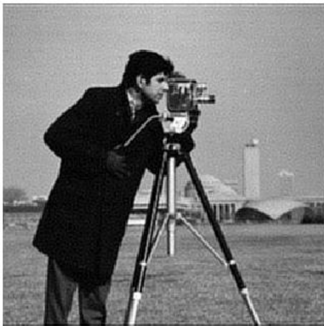
Figure 55: Result of Figure 4 restored by the iterative Tikhonov-Miller algorithm after 40 iterations, \alpha = 10^{-3} , ISNR = 2.73 dB
