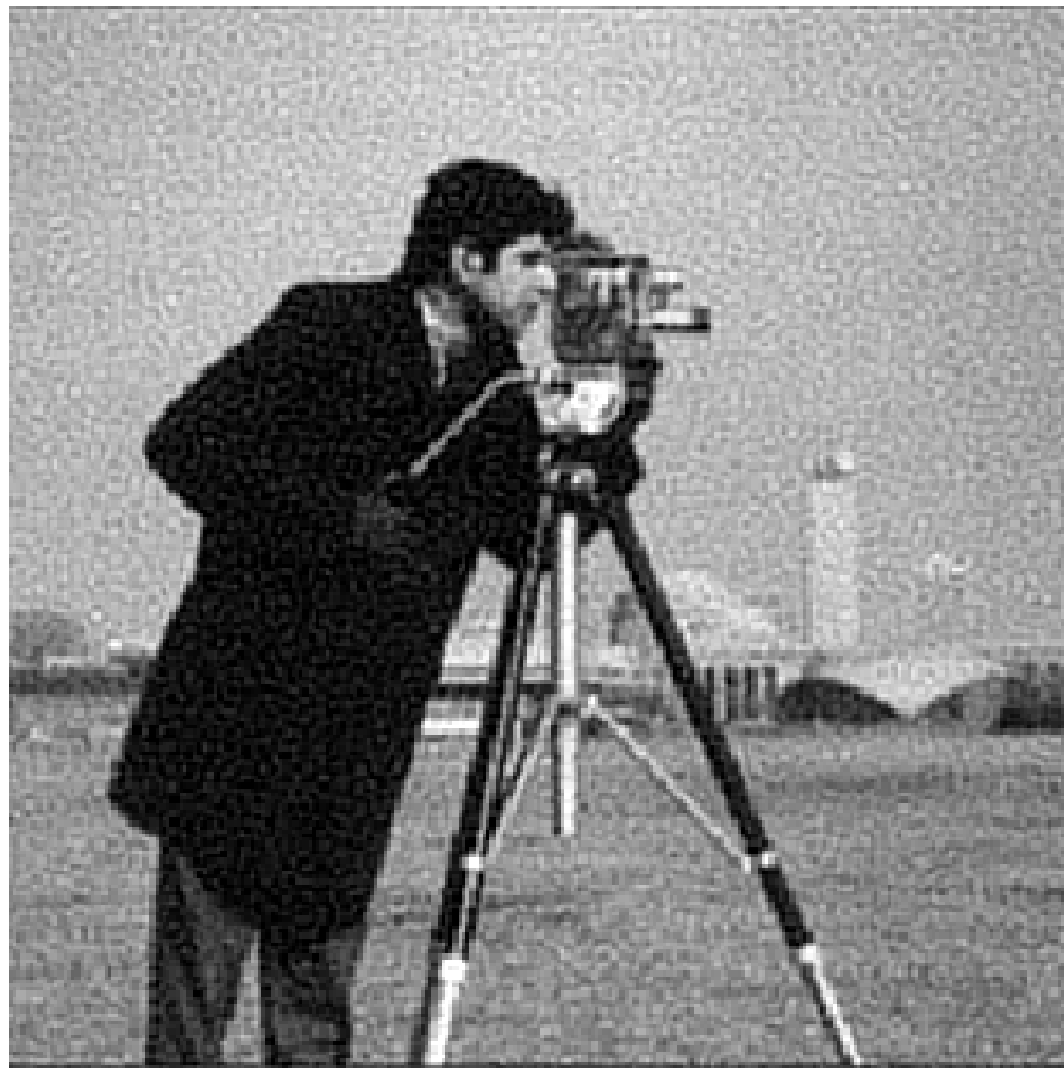
Figure 57: Result of Figure 5 restored by the iterative Tikhonov-Miller algorithm after 20 iterations, \alpha = 10^{-2} , ISNR = -2.70 dB
