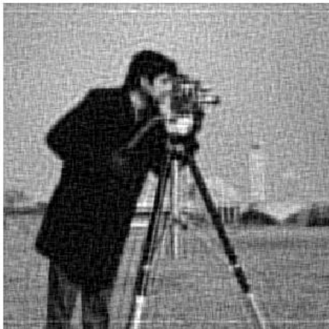
Figure 52: Result of Figure 3 restored by the iterative Tikhonov-Miller algorithm after 30 iterations, \alpha = 10^{-2} , ISNR = 1.42 dB
