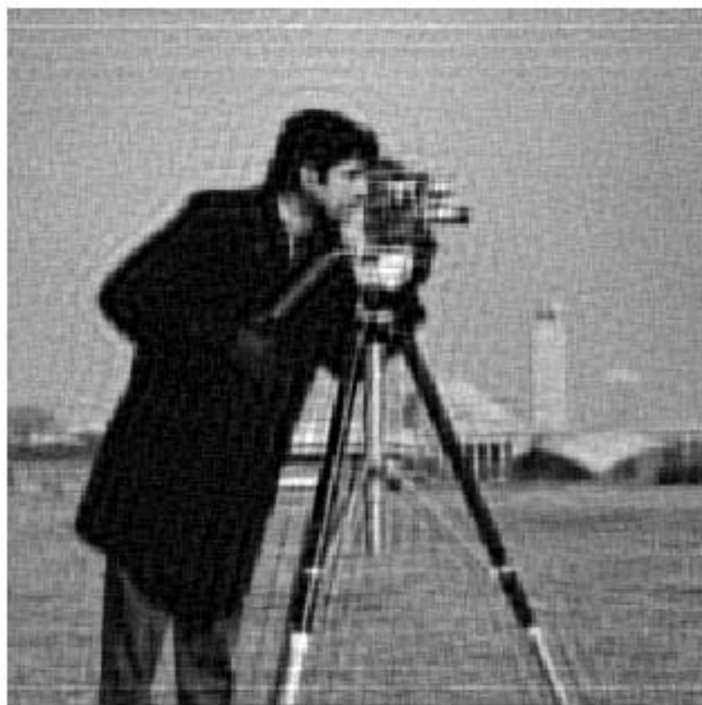
Figure 50: Final result of Figure 2 restored by the iterative Tikhonov-Miller algorithm (74 iterations), \alpha = 10^{-3} , ISNR = 4.15 dB
