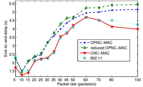
Fig. 8. End-to-end delay vs. packet rate in the #-shaped topology.
