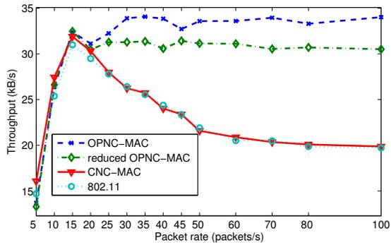
Fig. 7. Throughput vs. packet rate in the #-shaped topology.
