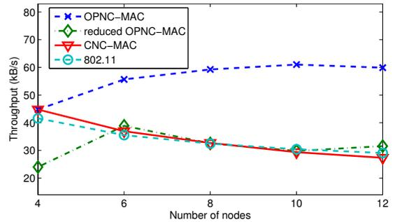
Fig. 5. Throughput vs. number of nodes in the wheel topology.
