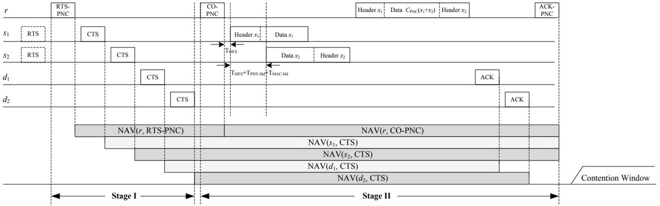
Fig. 2. Standard timing diagram of packet exchange in OPNC-MAC.
