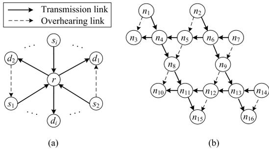
Fig. 4. Simulation topologies: (a) wheel topology, (b) #-shaped topology.
