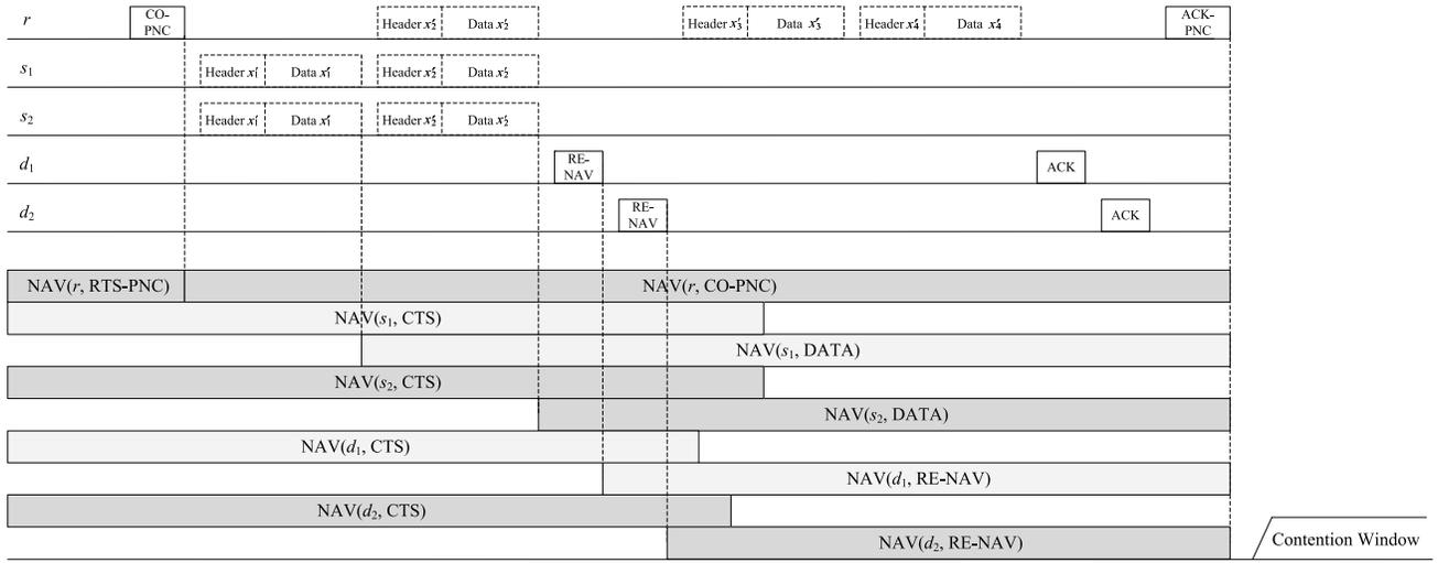
Fig. 3. Timing diagram of packet exchange in exceptional cases.
