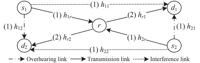
Fig. 1. Overhearing PNC in “X” topology. The number in the brackets indicates the communication phase.
