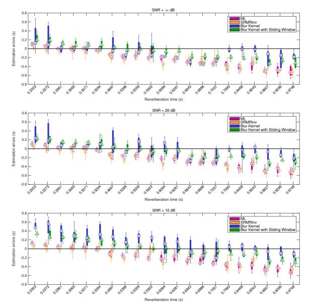
Figure 2: Estimation errors for the four algorithms compared, as a function of  $T_{60}$  and for different SNRs. The black dots denote the median, the thick vertical lines show the interquartile ranges and the thin vertical lines indicate the range up to 1.5 times the interquartile range.
