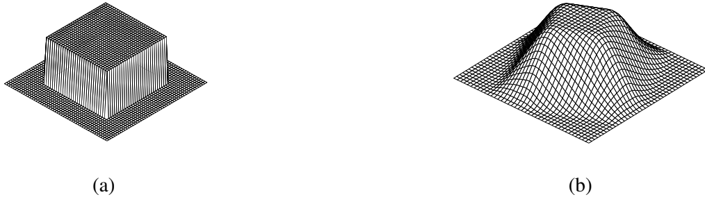
Fig. 4. Original and directional kernels: (a) \varphi_{xy}(x, y) is a Haar scaling function with support 1 \times 1 , (b) Directional kernel \zeta_{\theta_1, \theta_2}(x, y) with support 4 \times 4 for a given corner point of the polygon g(x, y) formed by the two sides with orientations \tan(\theta_1) = 2/1 and \tan(\theta_2) = -1/2 .
