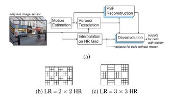
**Fig. 2**. (a) Deconvolution-based motion-deblurring on an adaptive image sensor. (b, c) Multiplexed LR and HR pixels of a hybrid grid.
