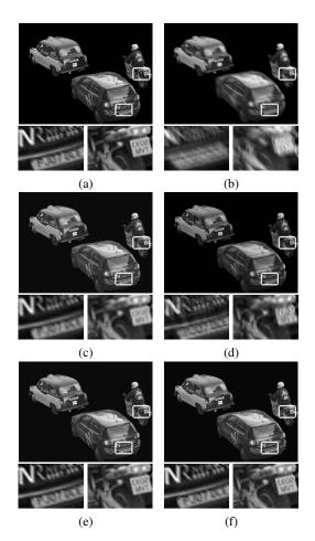
**Fig. 4**. (a) Ground-truth frame. (b) Blurred output for HR spatial resolution. (c) Bicubic interpolation of reference LR frame. (d) Output of deconvolution-based motion deblurring. (e, f) Output of SR-based deblurring after 10 (e) and 30 (f) iterations of the algorithm.
