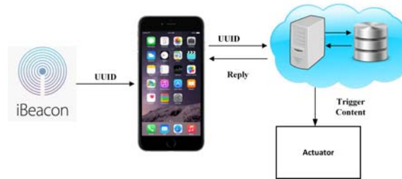
Figure 2.3. Working principal of the beacon
