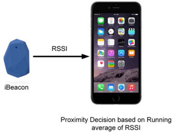
Figure 4.1. Current approach used by Apple's CoreLocation Framework.
