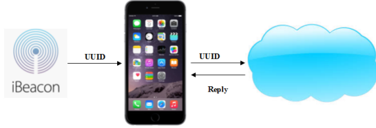
Fig. 1. Working principal of the iBeacon
