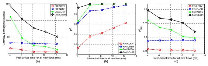
Fig. 2. The effect of network traffic on (a) Network Throughput, probability of successful end-to-end packet reception in terms of (b) Packet Delay and (c) PER.
