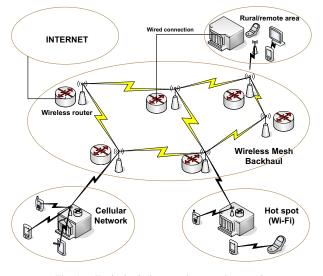
Fig. 1. Typical wireless mesh network scenario.
