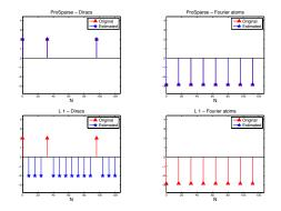
N = 128, K = 11, BP fails because it requires K = 10. Note: Counter example based on Feuer-Nemirovsky work. Simulation results courtesy of Jon Onativia Bravo (ICL).
