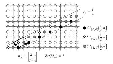
Fig. 8. The intersections between the 3 cosets of the lattice  $\Lambda$  given by the generator matrix  $\mathbf{M}_{\Lambda}$  and the digital lines  $L(r_1 = 1/2, n)$ , where  $n \in \mathbb{Z}$ , are the co-lines  $CL_{[0,0]}(1/2, n)$ ,  $CL_{[0,1]}(1/2, n)$ , and  $CL_{[1,1]}(1/2, n)$ .
