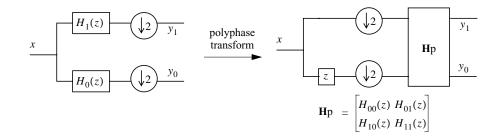
Fig. 11. A 1-D filter-bank  $(H_0(z), H_1(z))$  with the subsampling factor 2 is represented in the polyphase domain with the corresponding polyphase components  $H_{00}(z)$ ,  $H_{01}(z)$ ,  $H_{10}(z)$ , and  $H_{11}(z)$ .
