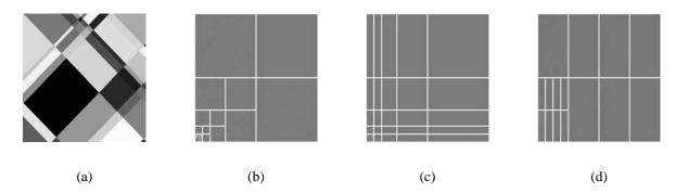
Fig. 6. (a) An example of an image from the class S-Mondrian( $\mathbf{M}(r_1, r_2), k_1, k_2$ ), for  $\mathbf{M} = [\mathbf{v}_1, \mathbf{v}_2]^T$ , where  $\mathbf{v}_1 = [1, 1]$  and  $\mathbf{v}_2 = [-1, 1]$ . The image is transformed using (b) S-WT, (c) S-FSWT, and (d) S-AWT( $\mathbf{M}_{\Lambda}, 2, 1$ ) (directionlets), where all the transforms are built on the lattice  $\Lambda$  determined by the generator matrix  $\mathbf{M}_{\Lambda} = \mathbf{M}(r_1, r_2)$ .
