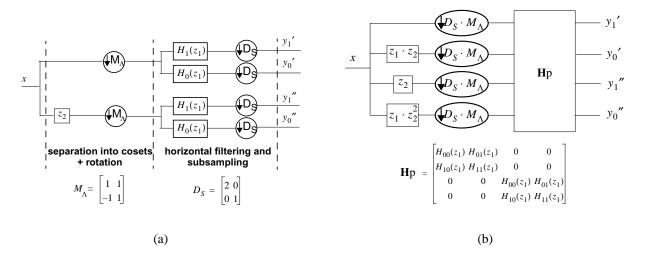
Fig. 12. (a) The 2-D two-channel filter-bank applied in the example shown in Fig. 9(a). Filtering and subsampling are applied in 2 cosets separately. (b) Equivalent polyphase representation contains 4 components. The polyphase transform  $\mathbf{H}_{p}$  is block-diagonal.
