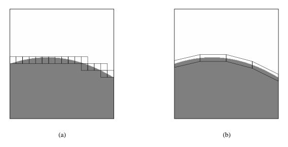
Fig. 2. A simple image with one discontinuity along a smooth curve is represented by the two types of basis functions: isotropic and anisotropic. The support of these basis functions is shown schematically as black rectangles. (a) Isotropic basis functions generate a large number of significant coefficients around the discontinuity. (b) Anisotropic basis functions trace the discontinuity line and produce just a few significant coefficients.
