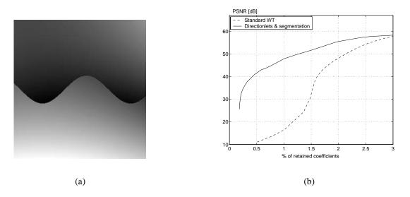
Fig. 13. An example of NLA of an image from the class  $C^2/C^2$ . (a) An image from the class  $C^2/C^2$  is approximated using the standard WT and the S-AWT( $\Lambda$ ,2,1) with spatial segmentation. (b) The MSE expressed in terms of PSNR is significantly reduced in the case of the S-AWT( $\Lambda$ ,2,1).
