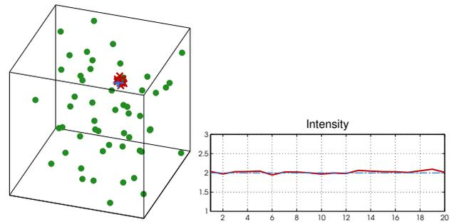
**Fig. 2.** Single point source recovery in 3D using samples obtained by  $N = 57$  sensors with  $K_1 = K_2 = 1$  for the spatial sensing function family  $\{\Psi_{\mathbf{k}}(\mathbf{x}) = e^{k_1(x_1 + jx_2) + jk_2 x_3}\}_{\mathbf{k}}$ .
