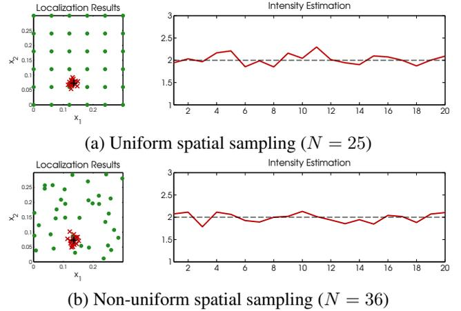
**Fig. 1.** Single source recovery for 2D Laplace field from spatial samples. Here  $K_1 = K_2 = 10$  for the spatial sensing function family  $\{\Psi_{\mathbf{k}}(\mathbf{x}) = e^{jk_1 x_1 + jk_2 x_2}\}_{\mathbf{k}}$ .
