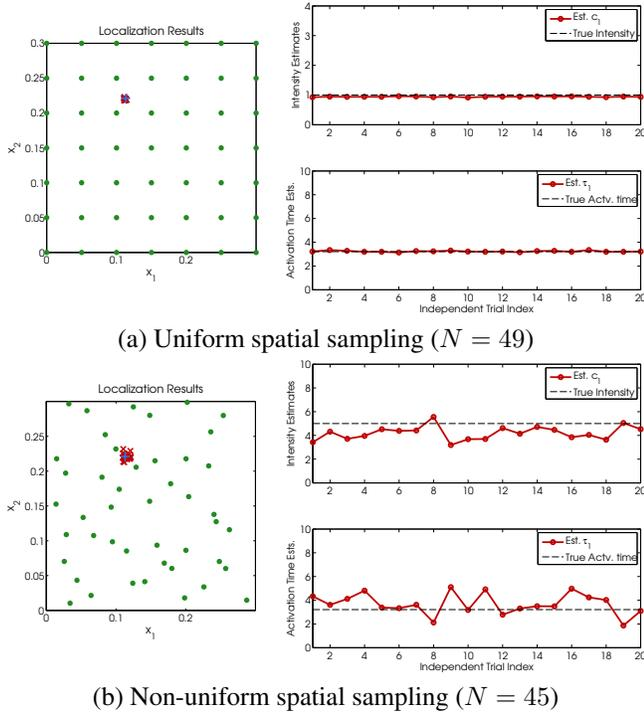
**Fig. 3.** Single source recovery from 2D diffusion field samples. Here  $K_1 = K_2 = 10$  for the spatial sensing function family  $\{\Psi_{\mathbf{k}}(\mathbf{x}) = e^{jk_1x_1 + jk_2x_2}\}_{\mathbf{k}}$  with  $k_2 = jk_1$ .
