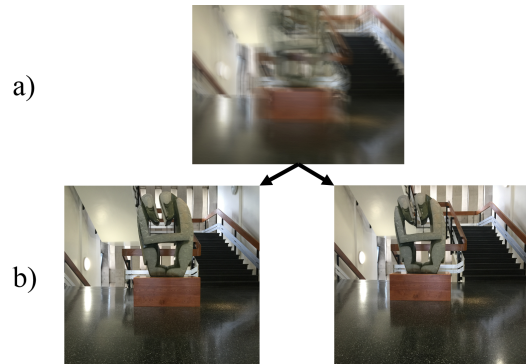
Fig. 1. a) shows a swiped image created by opening the camera shutter as the camera moves. b) shows the images reconstructed using the plenoptic function recovered from a).
