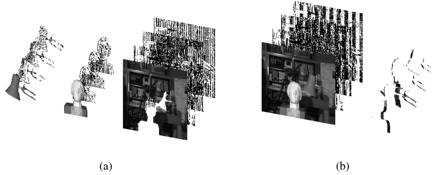
Fig. 8. (a) Tsukuba transform coefficients following the inter-view transform. Each transformed layer is composed of one low-pass subband and three high frequency images. (b) Recombined layers. The view subbands from each layer are grouped into a single image to increase the number of decompositions that can be applied by the spatial transform. Note that additional pixels must be transmitted to correctly reconstruct the layers at the decoder. A shape-adaptive implementation is used to efficiently deal with the irregular boundary of the occluded data.
