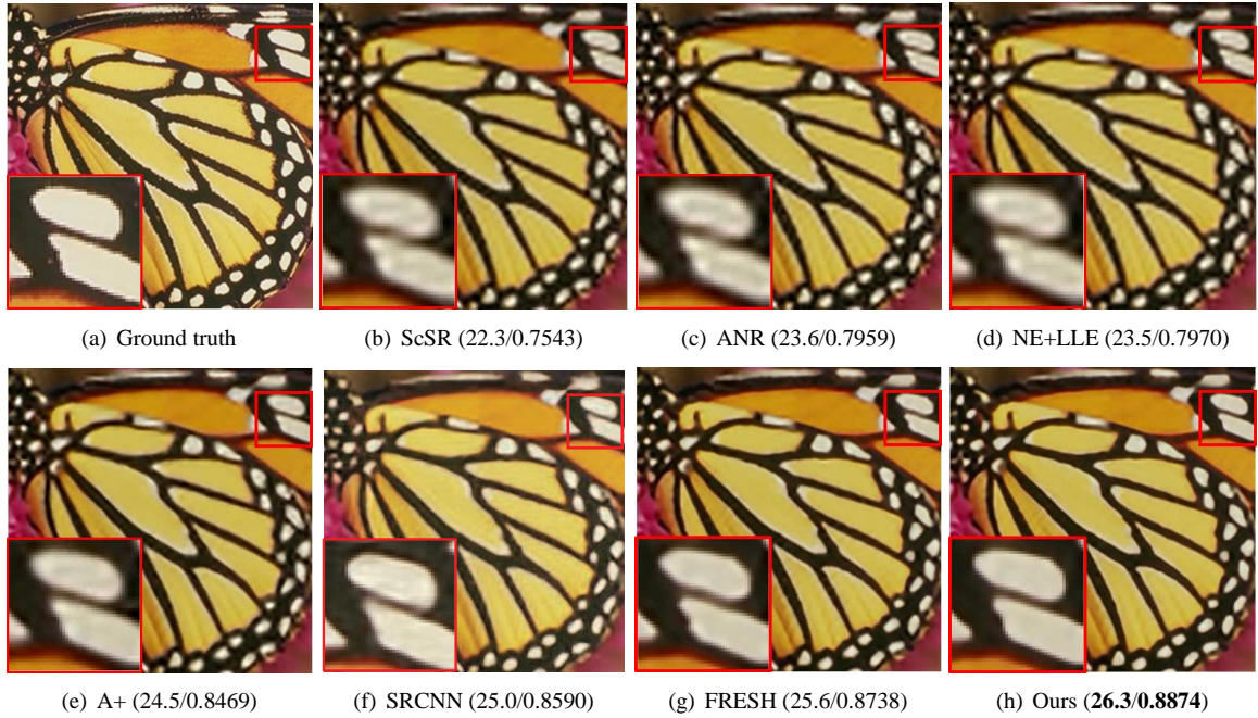
Fig. 3. SISR results of Butterfly by our and other methods with 4\times upscaling. The values in the bracket are PSNR/SSIM.
