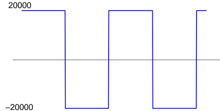
Sketch FM and PM signals if the modulating signal is the one above (on the left). The constants  $k_f$  and  $k_p$  are  $2\pi \times 10^5$  and  $10\pi$ , respectively, and the carrier frequency  $f_c = 100MHz$ .
