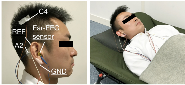
FIGURE 3. Recording setup in our study. Left: The electrodes were placed on scalp and ear. Right: The subject reclined in a comfortable chair.
