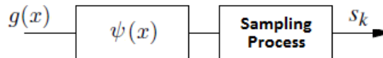
Figure 4.1: A system identification problem setup. Here, g(x) represents the continuous-time input signal, \psi(x) represents the unknown system and s_k represent the output samples
